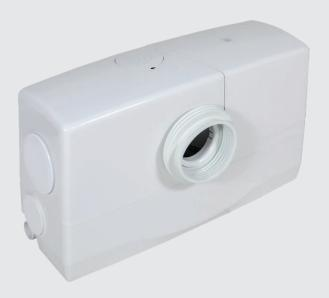
The PowerFlush Pro is a fully automatic macerator suitable for pumping waste from a complete bathroom to a higher level when gravity drainage is not possible and/or economical to install. The system can accept waste connections from a toilet, basin, shower or bidet. It is not suitable for connection to washing machine, dishwasher or bath.
