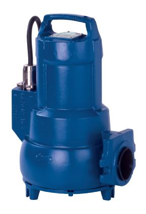
The state of the art Ama-Porter 502ND is designed for high operating reliability and is designed to give top performance due to a generously sized motor, thermal overload protection. The pump comes in a manual, automatic, single and three phase versions.
