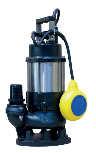
The JS250SV submersible sewage vortex impeller pump allows soft solids suspended in water to be passed through the pump body to waste. Supplied as standard as a free standing motor. The pump can be supplied with a conventional ball type 'MAC 3' float, fixed magnetic canister 'AGMA' float, or without a float for manual operation. Supplied free standing for quick installation.
