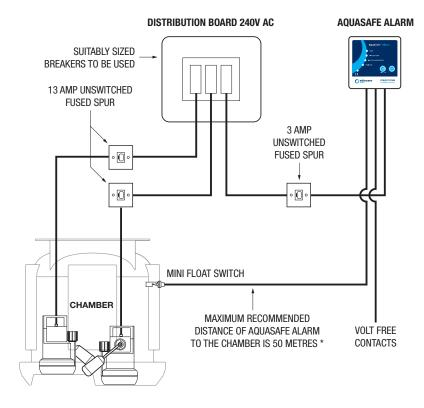
\* The float comes with a 5m cable. A cable extension and junction box (not supplied) is required if the alarm is installed more than 5m from the base of the chamber.
