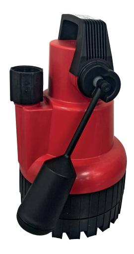
The state of the art EA33 is designed to give top performance and achieve high levels of efficiency thanks to optimised hydraulic systems and motors. The pump is fitted with a magnetic float switch with variable level control and maximum travel stop. A locking disk enables straightforward adaption of the pump to external control systems. Supplied free standing for quick installation.
