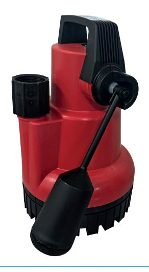
The state of the art EA31 is designed to give top performance and achieve high levels of efficiency thanks to optimised hydraulic systems and motors. The pump is fitted with a magnetic float switch with variable level control and maximum travel stop. A locking disk enables straightforward adaption of the pump to external control systems. Supplied free standing for quick installation.
