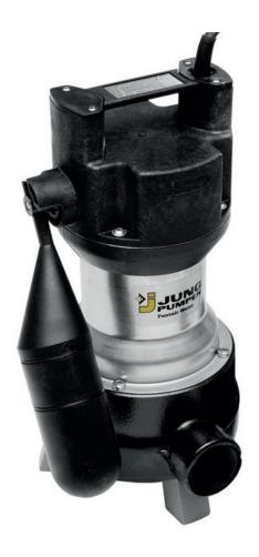
The heavy duty centrifugal submersible drainage pump US 73 HES is suitable for dealing with very contaminated water and capable of handling solids up to 30 mm particle size without stones. These pumps can be used wherever wastewater up to 90°C is involved, such as in laundries or automatic laundrettes, or in industrial dishwashers and washing machines or for the emergency overflow of heating systems. Can be supplied free standing, or pedestal mounted for permanent installations.
