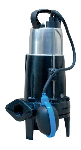
The Piranha 08 submersible pump offers problem-free pumping of sewage containing faecal matter. The pump has been designed for effective and economic dewatering using discharge lines of small diameter in private or domestic areas. The unique Piranha shredding system is suitable for cutting faecal matter. Can be supplied free standing, or pedestal mounted for permanent installations.
