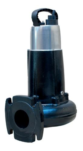
The MF665 submersible pump with a 60mm solids clearance offers reliable and effective dewatering. The compact shape and small sump requirements ensure a quick and cost effective installation of the pump. Easy Fit cable connector offers simple replacement of a damaged cable without disassembling the pump. Can be supplied free standing, or pedestal mounted for permanent installations.
