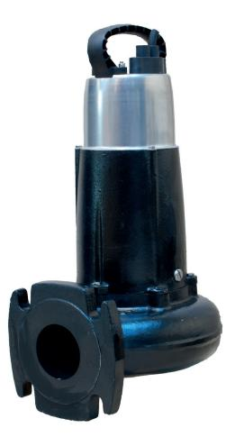
The MF565 submersible pump with a 60mm solids clearance offers reliable and effective dewatering. The compact shape and small sump requirements ensure a guick and cost effective installation of the pump. Easy Fit cable connector offers simple replacement of a damaged cable without disassembling the pump. Can be supplied free standing, or pedestal mounted for permanent installations.
