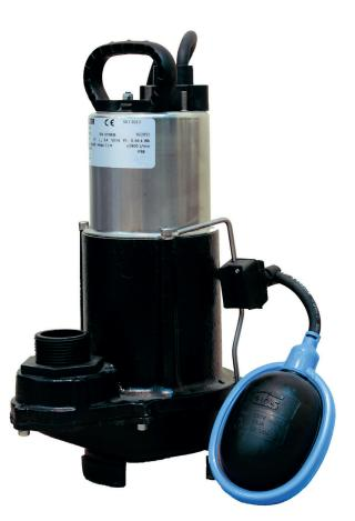
The MF154 submersible pump with a 20mm solids clearance offer reliable and effective dewatering. The compact shape and small sump requirements ensure a guick and cost effective installation of the pump. Easy Fit cable connector offers simple replacement of a damaged cable without disassembling the pump.
