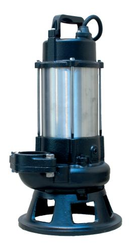
The JS750SK submersible sewage grinder impeller pump macerates soft solids suspended in water into smaller parts that can pass through the pump body to waste. Supplied as standard as a free standing motor, it can also be pedestal mounted for guide rail installation. The pump can be supplied with a conventional ball type 'MAC 3' float or without a float for manual operation.
