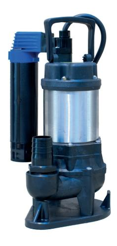
The JS150SV submersible vortex impeller pump allows soft solids suspended in water to be passed through the pump body to waste. Supplied as standard as a free standing motor. The pump can be supplied with a conventional ball type 'MAC 3' float, fixed magnetic canister 'AGMA' float, or without a float for manual operation. Supplied free standing for quick installation.
