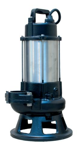
The HCP F-21 pump is precision manufactured utilizing the highest standard of quality control. It is offered as standard with epoxy resin sealed water resistant cable base, thermal motor protection and dual mechanical seal. Can be supplied free standing, or pedestal mounted for permanent installations.
