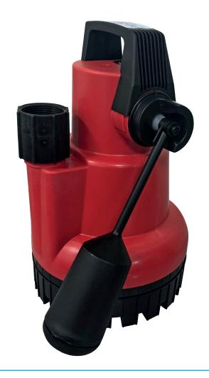
The state of the art Ama-Drainer 301 is designed to give top performance and achieve high levels of efficiency thanks to optimised hydraulic systems and motors. The pump is fitted with a magnetic float switch with variable level control and maximum travel stop. A locking disk enables straightforward adaption of the pump to external control systems. Supplied free standing for quick installation.
