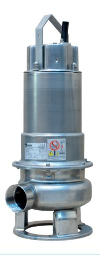
The DW150 VOX submersible pump is suitable for light screened Sewage and dirty water. The pump is manufactured entirely from a single sheet of 304 stainless steel. Comprising of a vortex impellor and incorporating a double mechanical seal. The volute of the DW150 VOX is made as an integral part of the pump casing using patented pressing technology. Can be supplied free standing, or pedestal mounted for permanent installations.
