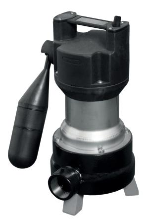
The heavy duty centrifugal submersible drainage pump US 73 HES is suitable for dealing with very contaminated water and capable of handling solids up to 30 mm particle size without stones. These pumps can be used wherever wastewater up to 90°C is involved, such as in laundries or automatic laundrettes, or in industrial dishwashers and washing machines or for the emergency overflow of heating systems. Can be supplied free standing, or pedestal mounted for permanent installations.
